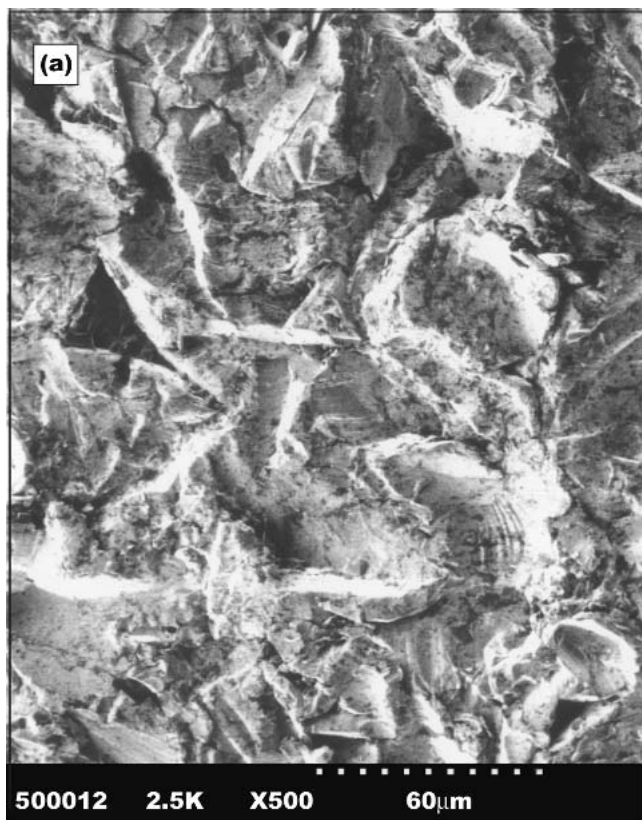
Fig. 3 Surface roughness morphologies of (a) uncoated and (b) coated HVOF aluminum coatings
